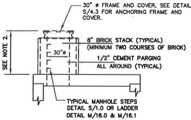
**MANHOLE FRAME AND COVER STACK DETAIL**
