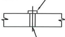
**LIFTING HOLE DETAIL**
