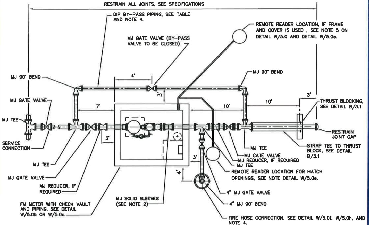
**PLAN - FM METER WITH CHECK VALVE IN VAULT
