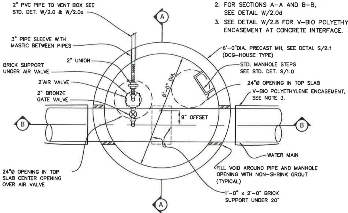
**AIR VALVE MANHOLE - PLAN**
