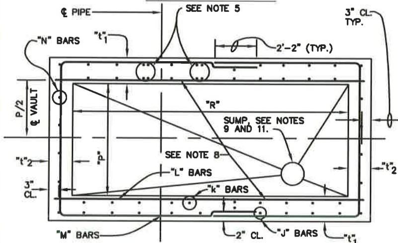
**PLAN-TOP SLAB REMOVED**
